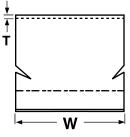
Tinnerman "U"-TYPE SPRING STEEL SPEED CLIPS Palnut Ρ Α **A1** w т Design Type: Industry Part Material Leg Length 2nd Leg Length Width Dual Barbs (B) or Number Thickness Panel Range Uneven Barbs (U) Ref Ref Ref Ref 22503-014 .015-.060 .50 .014 U .34 .34 20285-017 .050-.100 .34 .35 .017 В .50 в 5207-014 .060-.090 .34 .34 .50 .014 27091-014 .115-.185 .42 .42 .50 .014 В 43806-014 .170-.205 .43 .43 .50 .014 В 45931-014 .245-.255 .36 .50 В .36 .014
